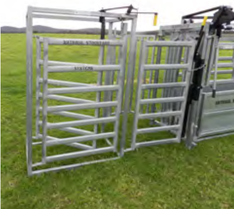
Rotate spring loaded handle to open off side gate. Locks over centre
