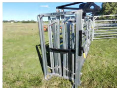
Basic Draft swivel posts fold back to give good head access
