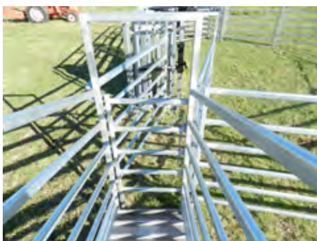
Basic Draft. Gates swing in unison. Push Pull one to work 2 gates. Swivel latch posts enable gates to be swung past the head of an animal after catching
