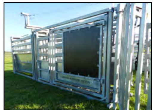
Weighing. Large weather proof EID antenna mounting board.
