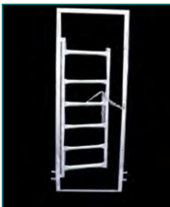
A common hinging and latching system. The double acting hinge which allows the gate to swing 360 degrees can suck back and leave a big gap between the post and the gate
