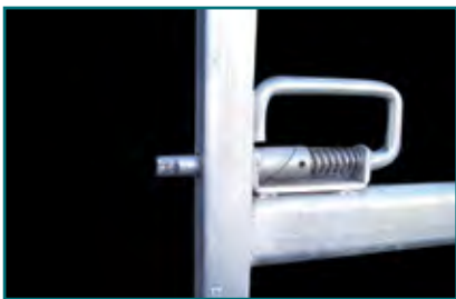
Slam catch pin does not rollback. Also easily opened by a tail bone, horn or nose due to no protective plate
